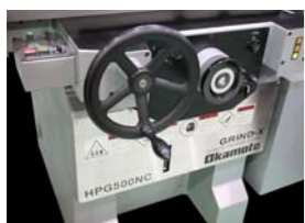
Longitudinal Cross feed handle *Standard Longitudinal handle is Round handle
