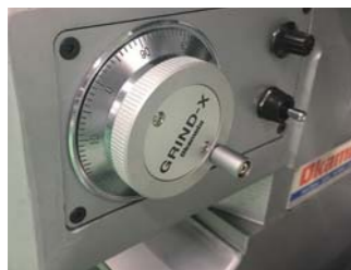
M.P.G. handle for Vertical infeed
