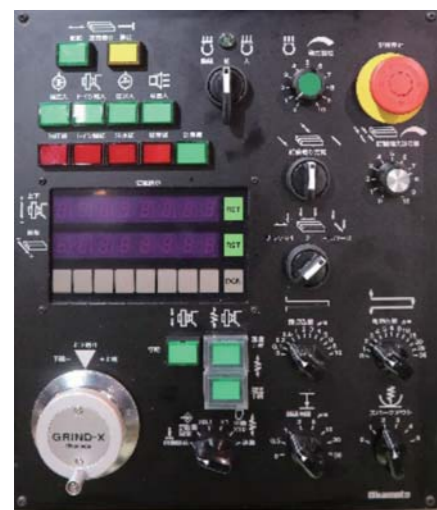
Operation panel for PFG500DXAL II *Standard operation panel is Silver color
