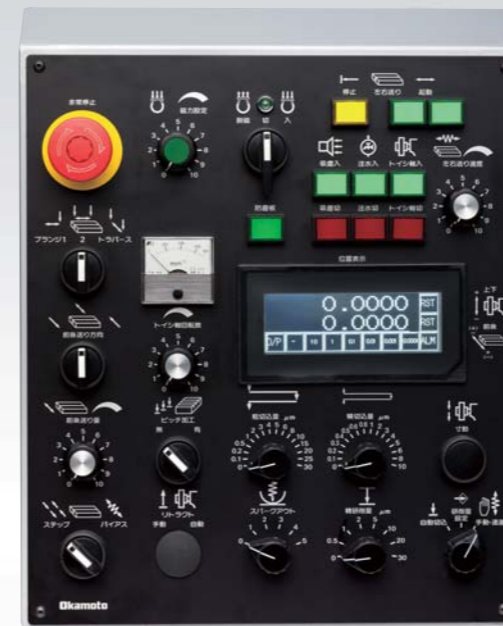
Operation panel for HPG500 model
