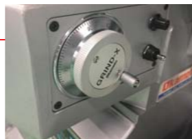
Vertical feed M.P.G. handle & jog feed switch's
