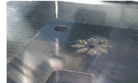
Hole diameter measurement of large dies
