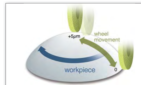
Complex Workpiece Workpiece that has corrugated shape in the center can be easily ground by CNC model.
