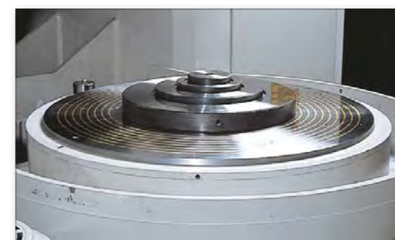
Steps Workpiece with multiple steps can be easily ground using the interactive software.
