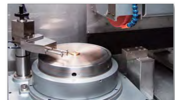
Ultra Precision Spacer (UPR3NC) Small workpieces that require ultra-precision flatness, such as bearing spacers for high-speed spindles can be ground.
